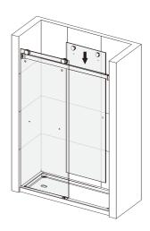
\*When installing the glass sliding door onto the sliding track, make sure that both wheels are correctly fitted to the sliding track and the glass is correctly fitted into the bottom fixer slot. Gently push the glass to check that it is sliding smoothly and also to ensure that it can be used safely.
