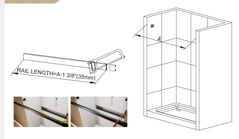
\*Measure the desired length and use a saw to accurately cut the aluminum to size, ensuring the edges are smooth and flat.
