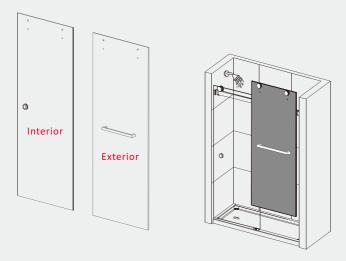
\* Place the finger pull glass on the *inside* of the shower enclosure where the shower head is located, and place the towel bar glass on the *outside* of the enclosure.
