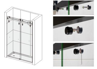
\*After ensuring the glass is level, install anti-jump nails to prevent the glass from accidentally falling and causing injury.
