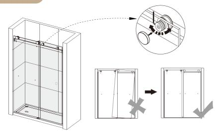
\*If you notice that the glass is not level at the top and bottom, adjust the eccentric screw on the wheels to ensure the glass is level.
