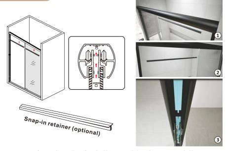
\*Optional anti-collision fixing buckles are provided to enhance a stronger hold.
