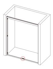
\*Position the guide block in line with the holes. Use a screwdriver to securely fasten the screws and place the cover.
