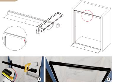
\*Measure the necessary length and use the cutting tool to precisely cut the stainless steel, ensuring a straight and accurate cut. Then, insert the cut track into the wall jamb's slot, ensuring it is level and vertical, and firmly secure it in place.
