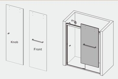
\* Place the Knob glass on the *inside* of the shower enclosure where the shower head is located, and place the towel bar glass on the *outside* of the enclosure.
